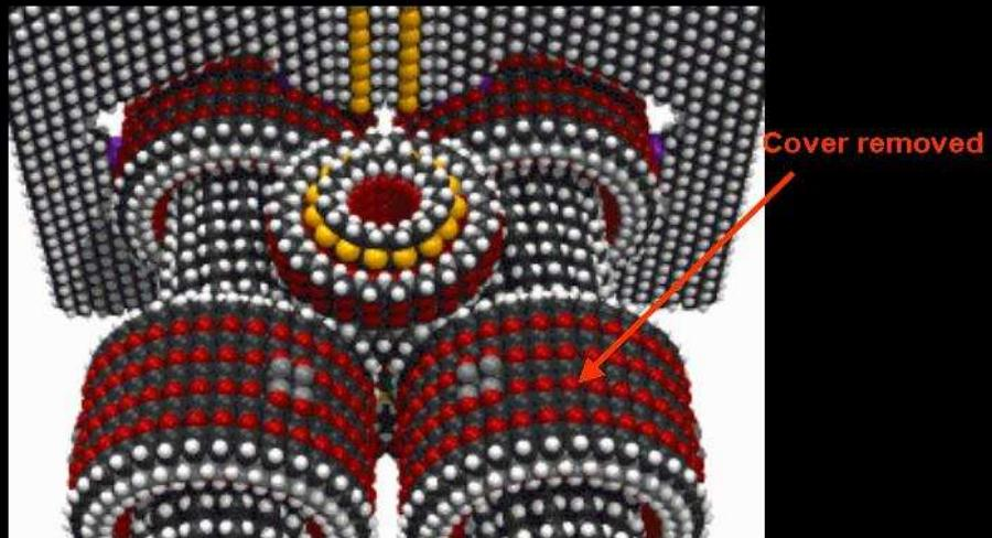
This worm drive assembly, designed by Dr Eric Drexler et al, includes 11 components totalling 25,374 atoms. It is the largest model ever simulated. More information about this coming soon. <sup>40</sup>
